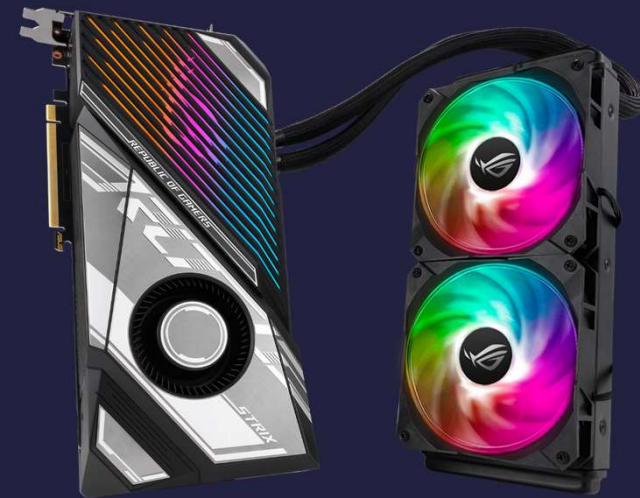
ROG Strix LC GeForce RTX™ 3080 Ti OC Edition with full-coverage cold plate cooling the GPU die and memory
